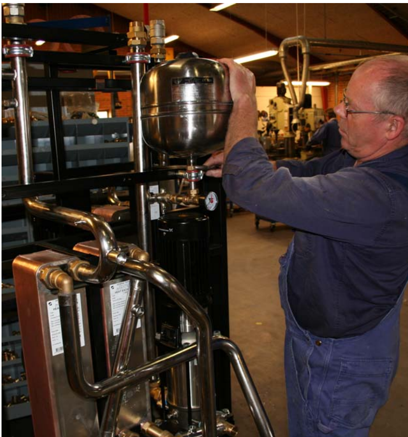
On the photo Bo Rasmussen from the forging department is mounting a cooling unit which is to be sent to a transmitting station in Hedensted
